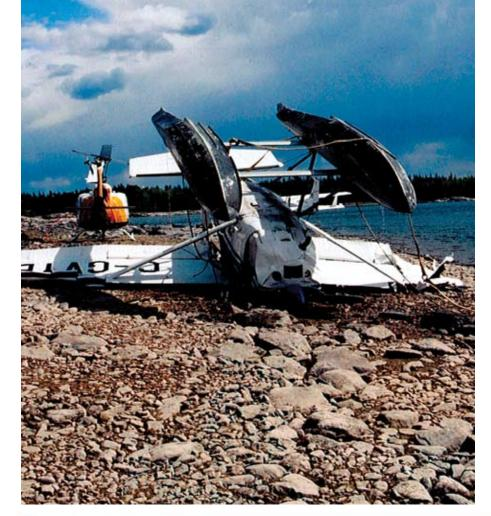
Battered but still basically intact, the airframe is typical of the condition of many floatplanes that upset. Surviving such a mishap is enhanced if passengers have basic knowledge of the action they need to take to get out.
